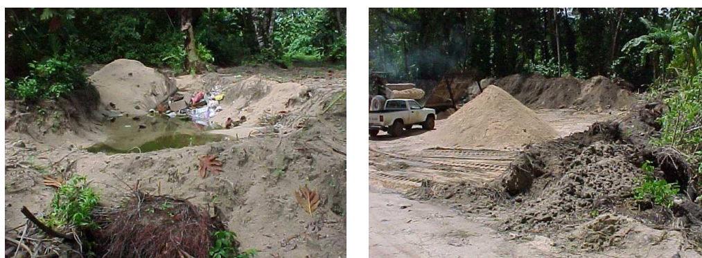
Figure 9: Typical small scale permitted sand mining site (left) and larger scale government site supplying sand for the hard sealing of the road between Okat and Walung.
